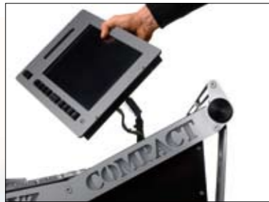
The Maxxyz Cerebrum module – like the other modules – is easily lifted from the frame
